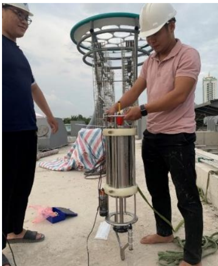
Figure 5. Using Midas-ECM and Levellogger Edge to measure flow velocity
