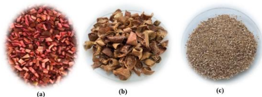
Fig. 1. Fresh (a) and dried (b), and finely ground peel waste (c) of purple passion fruit.
