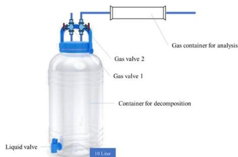
**Figure 1. Container design for composting**
