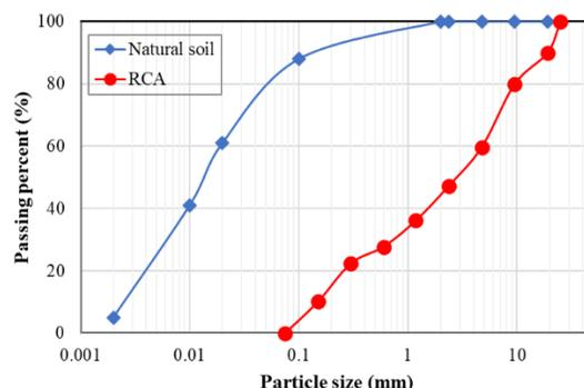
Figure 1. Grain size distribution curves for soil and recycled concrete aggregate
