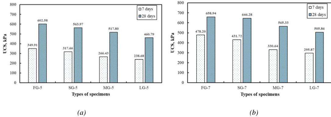
Fig 9. Effect of Curing Duration on UCS
