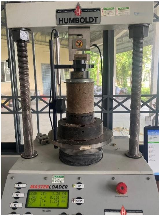
**Figure 5. Unconfined compressive test (UCS) apparatus**
