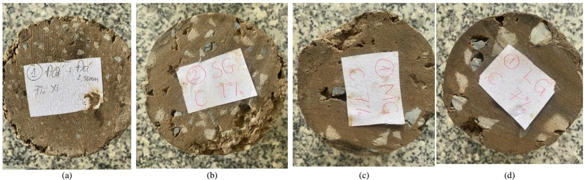
Figure 4. Cross-area of soil mixtures and RCA samples: (a) FG, (b) SG, (c) MG, (d) LG
