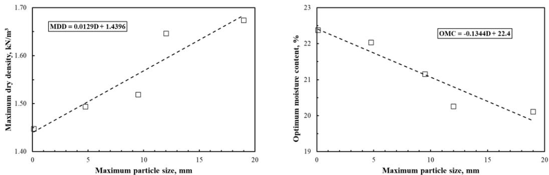
**Figure 7. The relationship between MDD, OMC, and particle sizes of mixtures**
