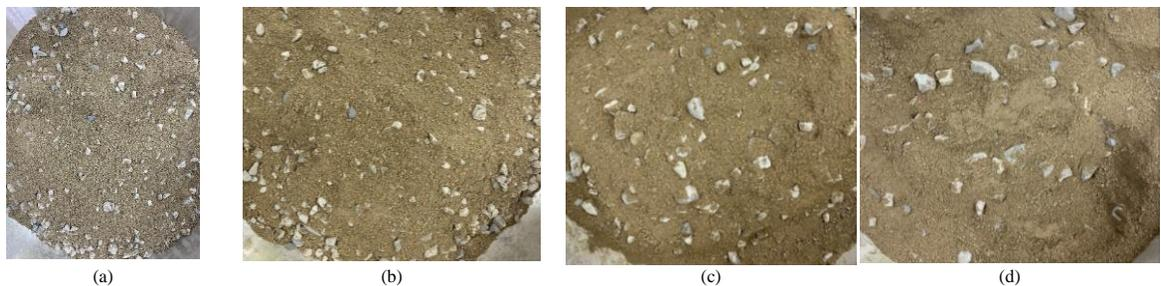
**Figure 2. Types of soil mixtures and RCA: (a) FG, (b) SG, (c) MG, (d) LG**
