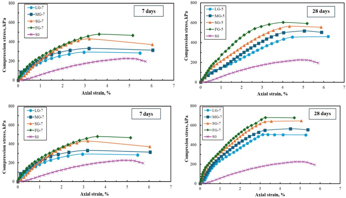
**Fig 8. Compression stress-strain curves of various SRCA blends at different curing periods**
