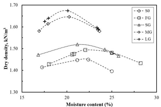
**Figure 6. Standard Proctor RCA and soil mixture tests**
