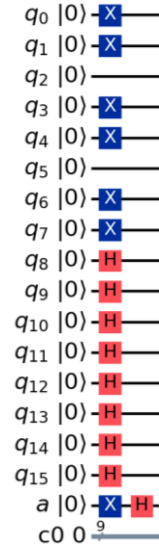
Fig. 7. Quantum circuit that implements steps 1 and 2 of Grover's algorithm
