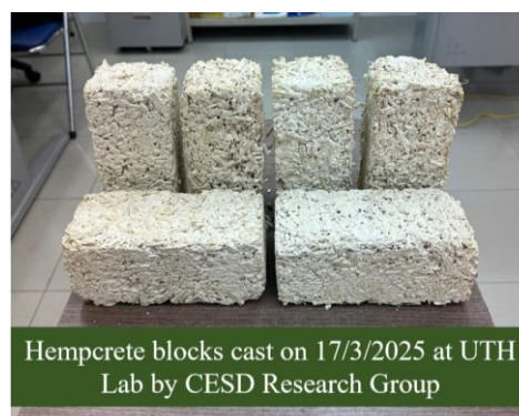
Figure 3. The hempcrete brick samples were cast by the CESD research team on March 17, 2025, at the Lab of the University of Transport in Ho Chi Minh City (District 12, Ho Chi Minh City)
