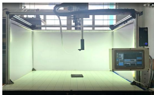
Figure 2. Experimental setup of the robot-vision system (3-axis robot, IMX219-200 camera with ring illumination, weld specimen, and NVIDIA Jetson Nano controller).
