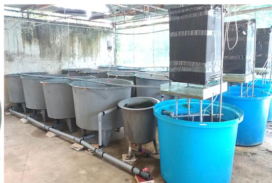
**Fig. 2: Experimental recirculation water system**
