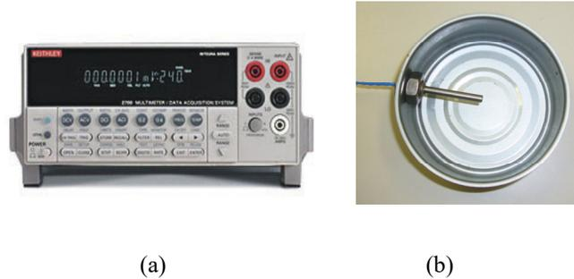
**Fig. 1: (a) Analog Keithley 2700; (b) Sensor position**
