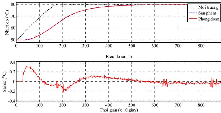
**Fig. 6: The output of the first order of transfer function model compared with the measured temperature response (above) and residual plot (below)**
