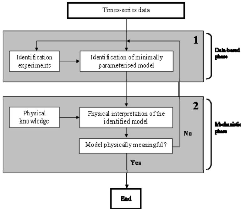
**Fig. 3: Data based mechanistic (DBM) modeling technique**
