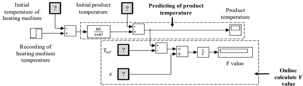
Fig. 7: The algorithm to predict product temperature during heating
