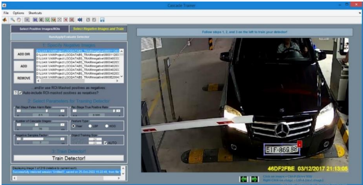
Figure 2. Choose regions of interest (ROI) for positive images and setup parameters in MATLAB's Cascade trainer tool
